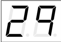
Activated when the PCM detects that any of the configurable output circuits is electrically shorted. This will only be detected whenever the output is powered. This is a non-critical fault and will not cause the heater to shut down. The output fault code refers to a specific hardware pin on the switch/control connector. (See wiring diagram on page 1-4.)
