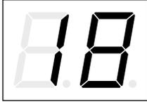
Indicates the heater was switched on via a CANbus input and then lost the CANbus heartbeat message for longer than 2 seconds.
