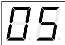
A VOLTAGE diagnostic code indicates that the supply voltage to the heater is out of the normal operating range for more than 10 seconds.
