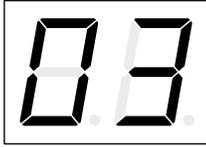
A COOLANT FLOW diagnostic code is displayed when the coolant temperature reaches 185°F (85°C) in less than one minute after ignition. This indicates that the coolant flow is severely restricted or blocked. This feature aids in detecting coolant flow problems that can degrade the PROHEAT performance.
