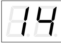
An HOUR METER (AUXILIARY OUTPUT) diagnostic code Indicates a short circuit fault in the harness or the device being operated by the Hour Meter (Auxiliary Output). This is a non-critical fault and will not cause the heater to shut down, heat to the engine will be maintained. An open circuit will not display a diagnostic code.
