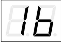
Indicates that the total system current limit of 15 amps was reached as measured by the PCM.
