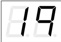
Indicates that the PCM's onboard temperature reaches 203°F (95°C).
