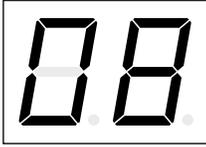
The FUEL PUMP diagnostics code is not used on the X45 Plus and indicates that the wrong configuration number was installed. See “CC” on page 4-6.
