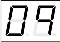
The COMPRESSOR diagnostic code is activated when the PCM detects that the compressor motor is electrically shorted, open, overloaded (software breaker hasn't tripped), or is damaged (compressor is running when it shouldn't be “ON”).
