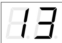
A SLEEPER FAN diagnostic code indicates an electrical short in the sleeper fan wiring harness, electrical connections, or fan motor. This is a non-critical fault and will not cause the heater to shut down, heat to the engine will be maintained. An open circuit will not display a diagnostic code.
