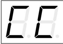
A configuration code is displayed if the PCM is powered up and no configuration number is set.
