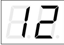
A BLOWER diagnostic code indicates an open circuit in the wire harness, a short in the wire harness between the positive and negative leads or an internal short in the motor.
