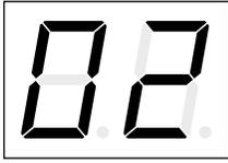
Indicates that a flame was detected (started successfully for at least 60 seconds) but is unable to maintain a steady flame before reaching the cycle off temperature of 185°F (85°C).
