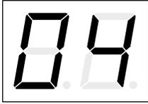
An OVERHEAT diagnostic code is displayed when the overheat breaker has tripped, shutting the heater down. This occurs if the heater has been started with little or no coolant and the heat exchanger temperature reaches 280°F +/- 12°F (138°C +/- 11°C).
