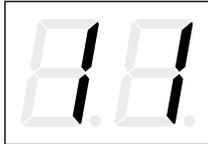
A COOLANT PUMP diagnostic code indicates an open circuit in the wire harness, a short in the wire harness between the positive and negative leads, an internal short in the motor, or an overload fault detected.
