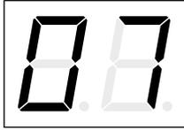
A TEMP SENSOR diagnostic code indicates a short or open circuit in the temperature sensor wiring or the coolant temperature is out of range—below  $-58^{\circ}\text{F}$  ( $-50^{\circ}\text{C}$ ) or above  $266^{\circ}\text{F}$  ( $130^{\circ}\text{C}$ ). The resistance of the temperature sensor is proportional to temperature.
